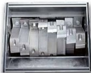
Cutting chamber of the MAS3 granulator model with 8 x 3 staggered knives.
