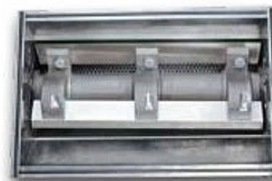
Cutting chamber of the MAS4 granulator model with 3 moving and 2 fixed knives.
